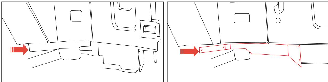
2. While holding the side panels in place position the supplied ATTICA's JK Wrangler Rear Center Fascia Cover Panel to ensure the outer panels and the center are aligned and spaced equally as shown in the image below.
