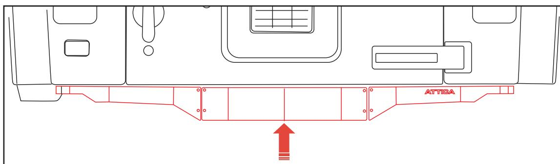
3. Mark the all hole locations in both the ATTICA's JK Wrangler Rear Driver, Passenger Side Fascia Cover Panels, and Rear Center Fascia Cover Panel carefully while holding all three panels in position to ensure the best fitment. This step is critical to ensure that the gap and panels are align when installed. Then remove all the panels and drill 8mm diameter holes at all the marked mounting locations.
