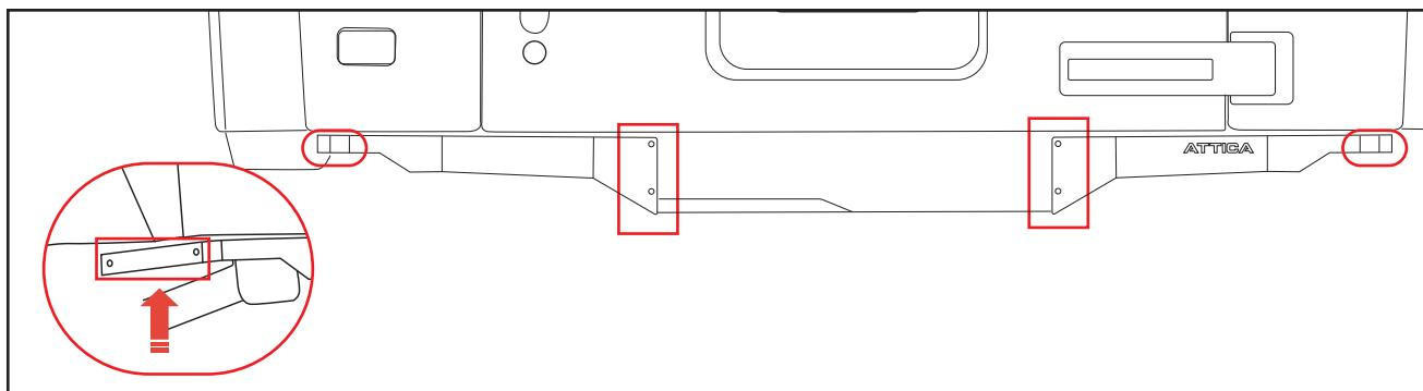
5. The Rear Center Fascia Cover Panel is secured using M8×20 hex socket button head bolts, flat washers, and hex flange nuts (place the flat washers on the same side as the nuts). There are 2 mounting points per side(4 in total).
