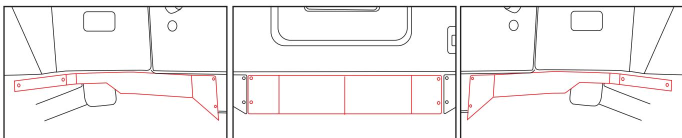
4. The Driver Side Fascia Cover Panel and Passenger Side Fascia Cover are secured using M8×20 hex socket button head bolts, flat washers, and hex flange nuts (place the flat washers on the same side as the nuts). There are 4 mounting points per side(8 in total).
