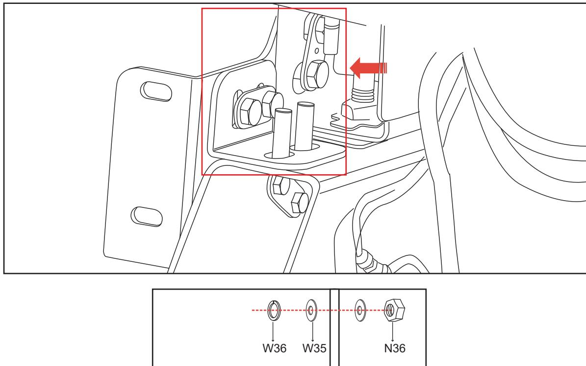
3. If your vehicle is a 2023–2025 F-250 / F-350, secure the brackets to the frame as shown by the arrows in the diagram using double screw plates, M10\*40 bolts, flat washers, spring washers, and nuts (a total of 4 mounting points on both sides).
