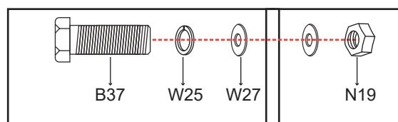
2. As shown by the arrows in the diagram, secure the brackets to the frame (a total of 12 mounting points on both sides).
