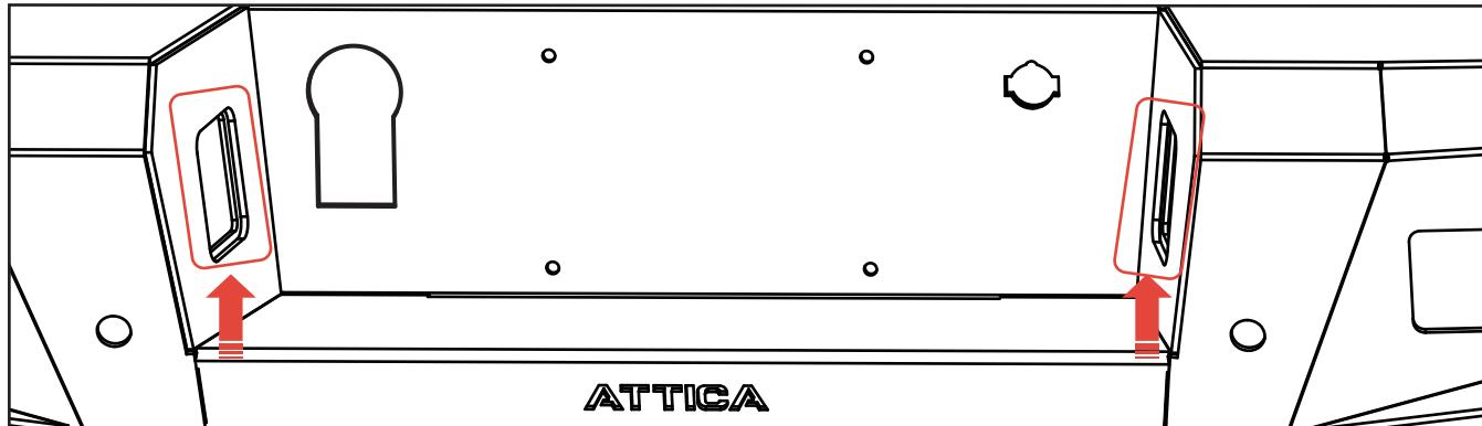
2. Install the factory sensors and trailer connector onto the rear bumper. Please note that the rubber sleeve must be trimmed according to the shape of the sensor, and then fitted over the sensor.
