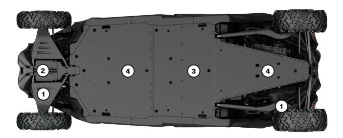
Our Plastic Plates glide smoothly and silently over obstacles, offering great protection in rough terrain. Made of abrasion-resistant thermoformed %" (10 mm) thick High Molecular Weight Polyethylene (HMWPE).
