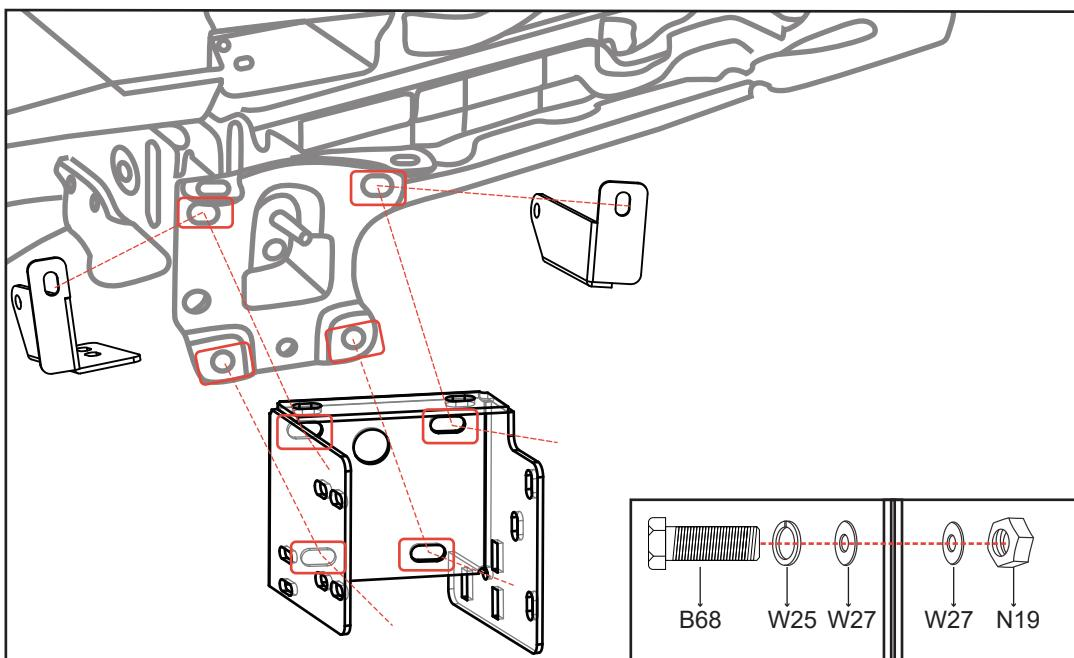
3. Install the ATTICA front bumper onto Bracket A.
