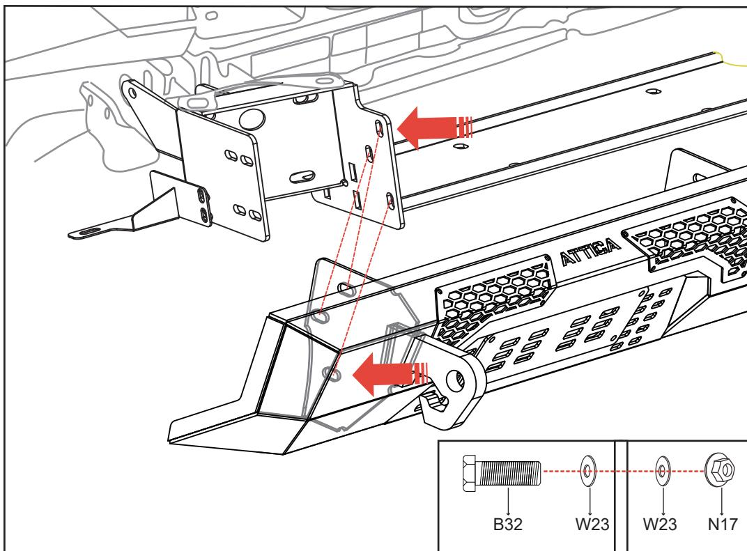
2. Secure Bracket C to Bracket A (1 per side). Then attach the factory fascia to Bracket C to prevent it from moving.
