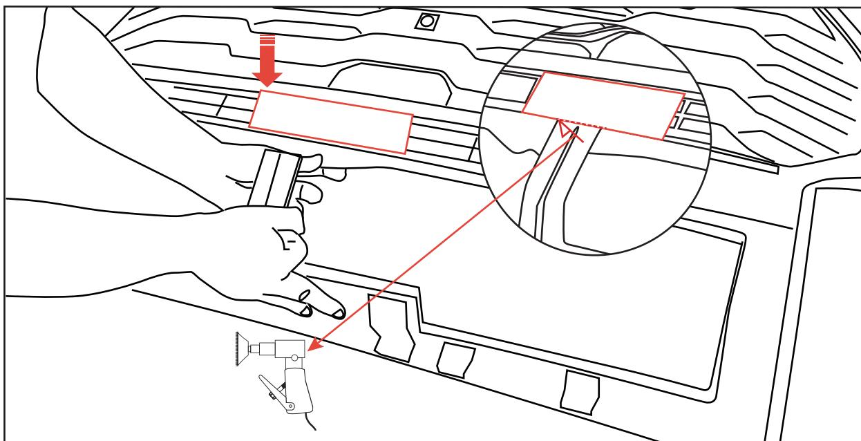
2.Next, make the cuts at the locations shown in the diagram on both the left and right sides. Then, remove the plastic pieces that were cut out.
