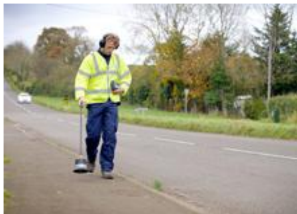
Detecting leaks using a ground microphone.
