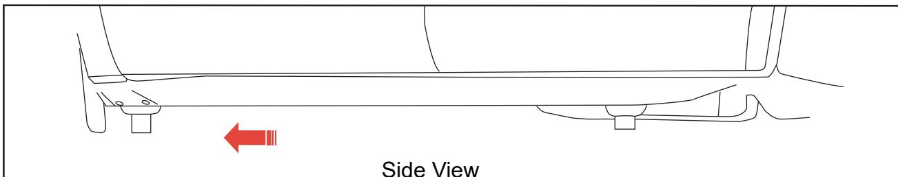
2. The arrow indicates the mounting hole on the vehicle. Attach the bracket to the vehicle's mounting hole.
