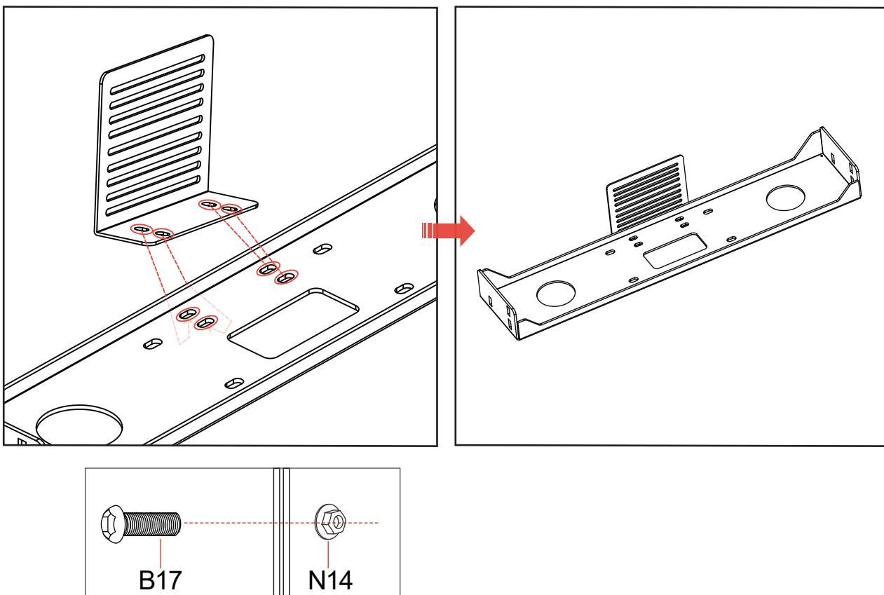
2. Secure the winch to the winch plate. Secure the control box to the winch control box relocation bracket, then mount the winch plate to the vehicle.
