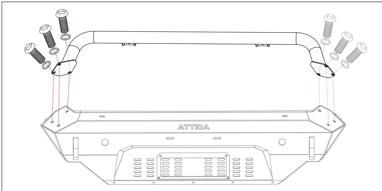
2. Assemble the main body with the side wings.
