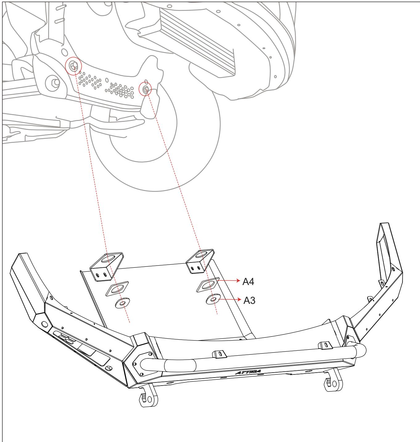
2. Install the skid plate brackets on the factory mounting points.
