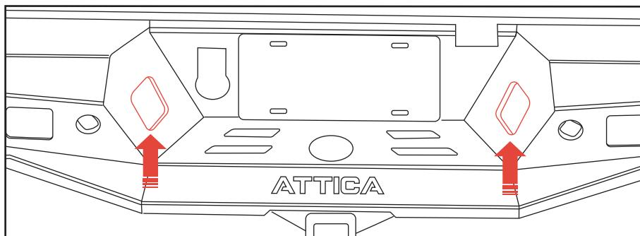
2. Install the factory sensors and trailer connector onto the rear bumper. Please note that the rubber sleeve must be trimmed according to the shape of the sensor, and then fitted over the sensor.
