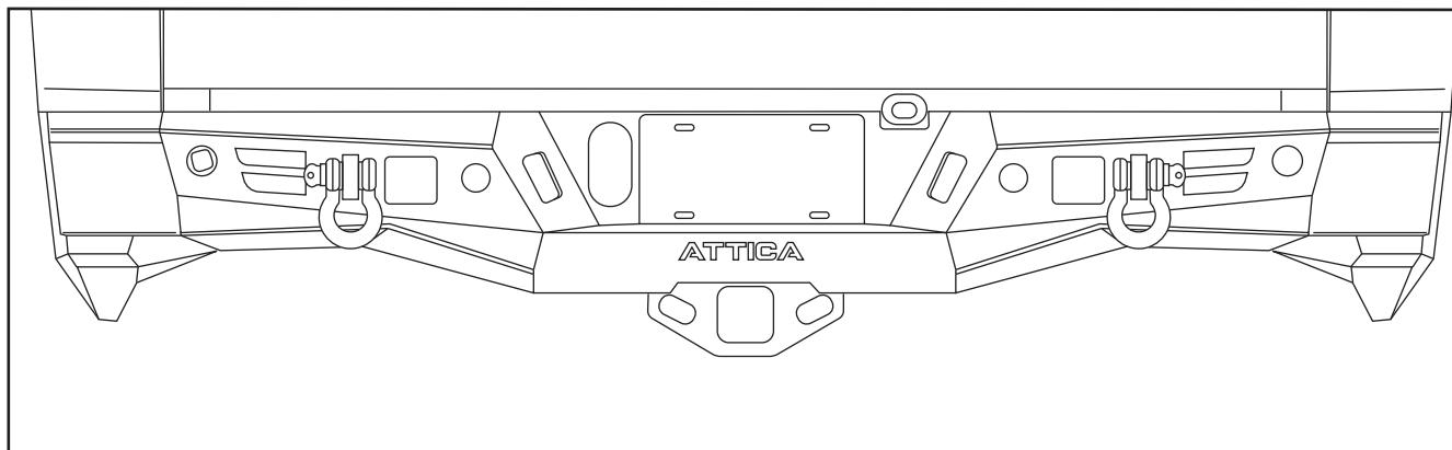
2. As shown in the diagram, secure the ATTICA rear bumper to the bumper brackets using M10x35 hex bolts (NO.B35), M10-8 hex nuts (NO.N15), φ10x25 flat washers (NO.W23) and φ10 spring washers (NO.W22). There are 2 mounting points per side (4 in total).
