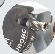
Cutter position at the cutter sharpening blade
